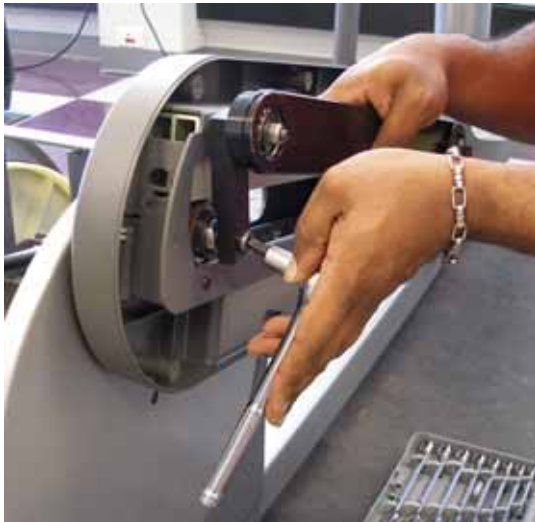
Fig. 9: attach the opposite end of the control link assembly Fig. 10: new control link assembly installed.
