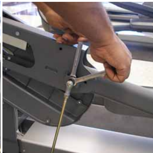
Fig. 6: removing the control link assembly
